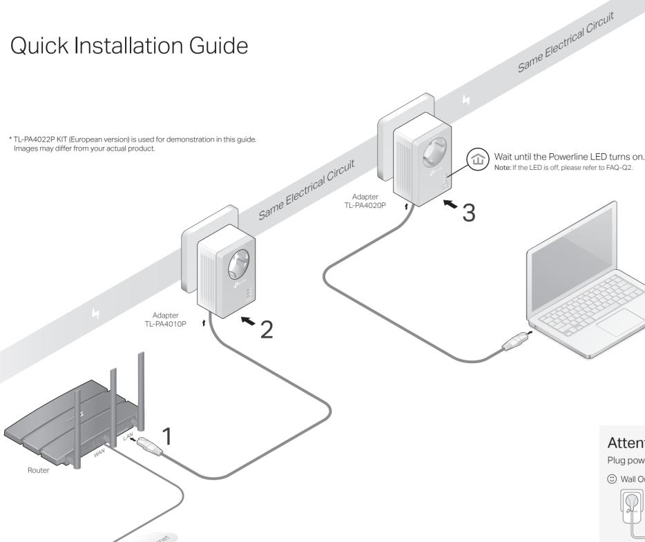
More: To add additional powerline adapters and extenders with the default settings, simply plug them into the wall sockets on the same electrical circuit.
